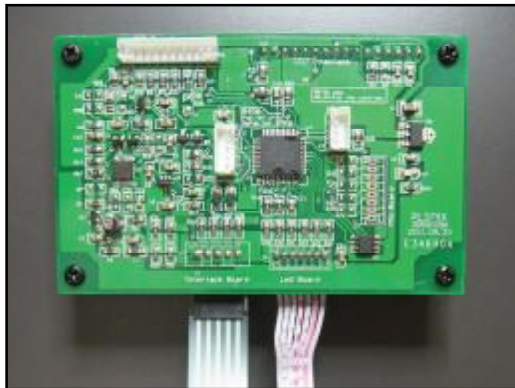
MCU Board is mounted behind the LCD display assembly on the front panel.
